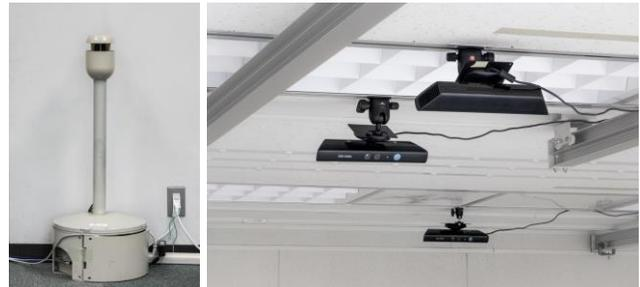
Figure 1. Left: Portable pole with laser range finder for 2D tracking system. Right: Ceiling-mounted 3D range sensors (Kinect) used for pedestrian tracking.
