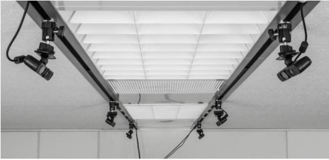
Figure 3. Arrangement of ceiling-mounted 3D range sensors (Asus). Sensors are inverted and mounted at an angle to maximize the coverage of the tracking system.
