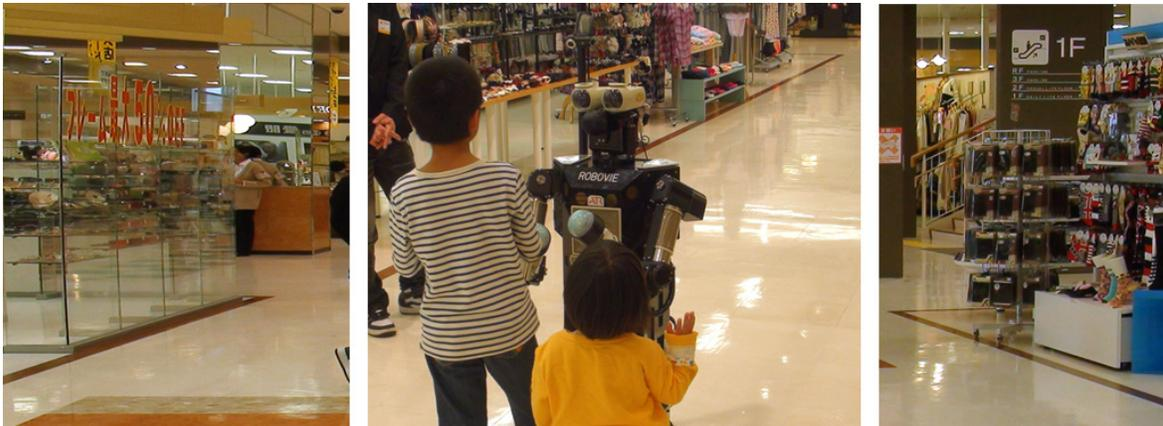
Figure 7.12: Dangerous areas in a shopping mall. Left: glass walls. Center: movable tables and shelves where only legs are visible to ground-level laser range finders. Right: movable clothing rack where only center pole is visible to laser range finder.
