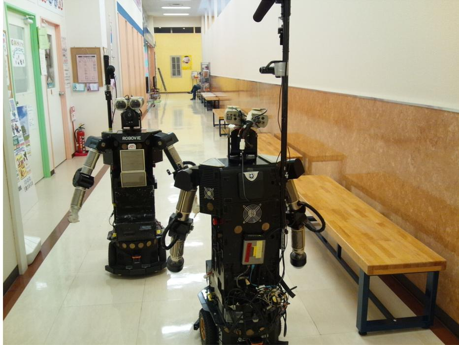
Figure 7.8: Deadlocked robots unable to pass each other in a corridor
