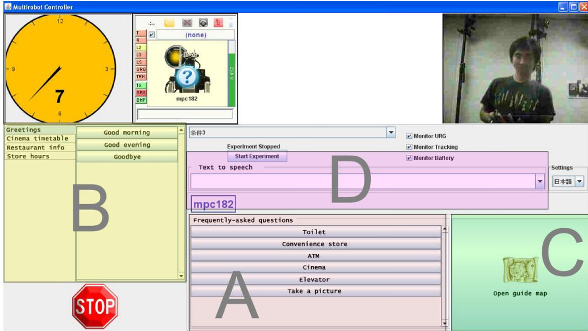
Figure 5.5: Screenshot of the teleoperation interface. The clock in the upper left was shown only for some conditions of the study presented in Sec. 5.6
