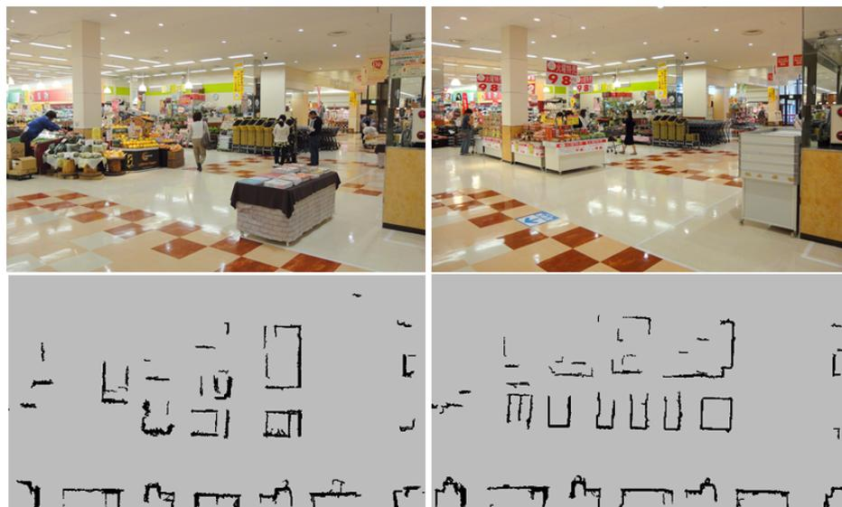
Figure 7.7: Example of an area in a shopping mall where features change from day to day. Top: photos on two different days. Bottom: laser scan maps of the area on two different days.
