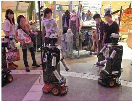
(b) Example of a robot mistaking another robot for a human and talking to that robot instead of an actual customer.
