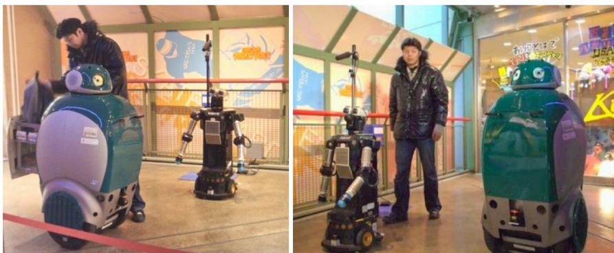
Figure 22. Collaboration between Robovie and DustCart, supported by the NRS.
