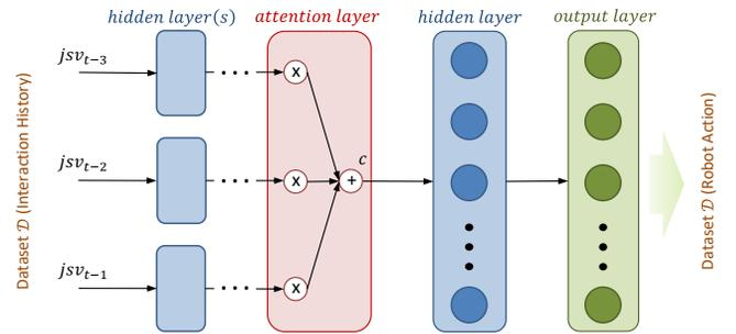
Fig. 2. Schematic of the multilayer perceptron neural network. Interaction history is inputted to the neural network as joint state vectors and robot action as training target for the neural network.
