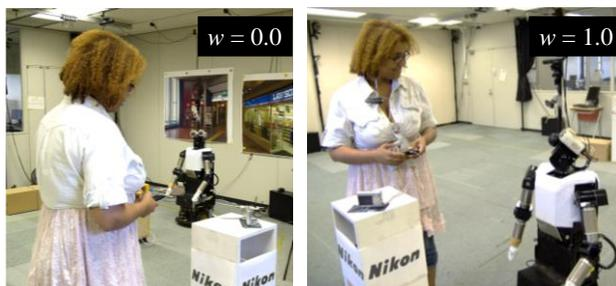
Fig. 4. When  $w = 0.0$ , the robot waits by the service counter as customer enters the shop. When  $w = 1.0$ , the robot approaches the customer as she enters the shop.
