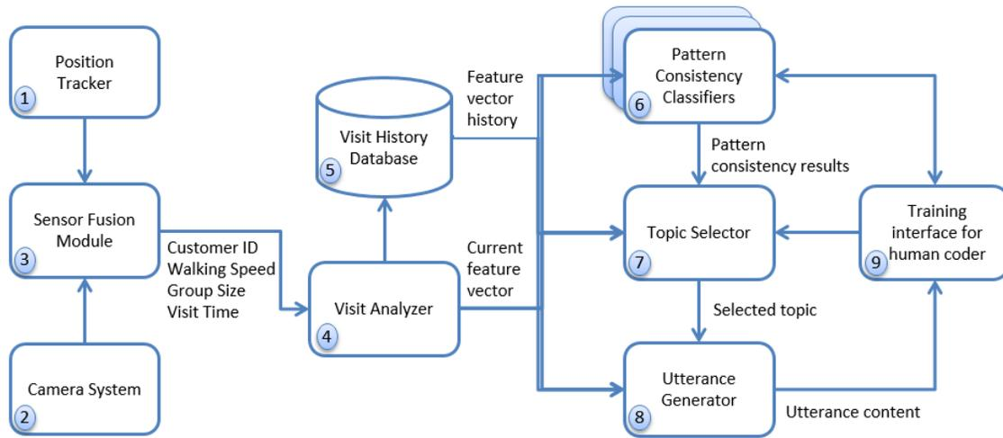
Figure 1. Data flow for training phase. System elements are numbered for reference in the text. Sensor data is used to generate feature vectors which are used as inputs to pattern consistency classifiers and topic selector. A human coder provides training data for the classifiers
