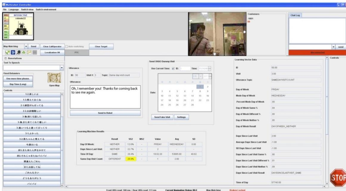
Figure 5. Graphical interface used by the operator. Video is shown on the upper center panel, buttons to trigger general utterances are presented on the left, and the panel in the center displays the greeting utterance generated by the system, which is sent to the robot when the operator clicks the button below it. The remaining displays show internal variables for the prediction system, which were only used for testing and debugging
