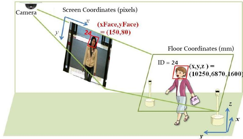
Figure 3. Illustration of sensor fusion between a camera and the position tracking system. The positions of people in the floor coordinate system detected by the position tracker are projected into the screen coordinates of the camera system. Nearest-neighbor matching is then used to associate face ID's with anonymous pedestrians detected by the tracking system
