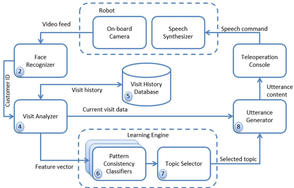
Figure 4. Architecture of the greeting system used in the field trial. Numbered elements correspond to elements presented in Fig. 1. Elements 1, 3, and 9 are not present here because the tracking system, sensor fusion, and training interface were not used in the field trial
